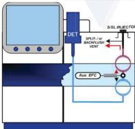
Deans switching enables the use of multiple traps and columns of differing phases in one method/analysis. It is the basis of two dimensional GC and many standard analyzers manufactured by Scion Instruments. Use our expertize to configure the optimum system for you.
